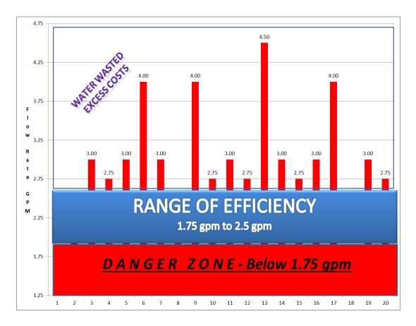
The chart above compares audited actual shower flow rates. The Range of Efficiency flow rates are 1.75 gpm to 2.5 gpm and the danger zone flow rates below 1.75 gpm.
